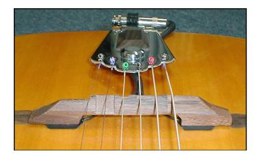
The cables can be hidden under the strings and the tailpiece. The ¾" adjustable rubber sleeve on the cables can be pulled tight towards the pickups to avoid mechanical cable noise.
