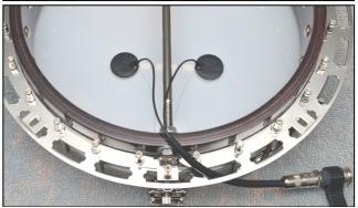
8. Remove the single dual-lock piece (the Velcro like black material around the jack). Save it along with the spare semi-circular foam pieces, gaping strips, and cable ties.
