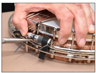
11. Secure the pickup cables with 2 cable-ties on the upper rod. This is VERY important as an unsecured cable will make noise that sounds like distortion or similar noise when plugged in. Make sure the cables from the pickups to the first cable tie are absolutely free in the air!
