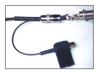
6. Solder as show in picture below: inner white conductor to ring terminal (medium length terminal of the 3 center terminals) and the blank ground conductor to the ground tab.
