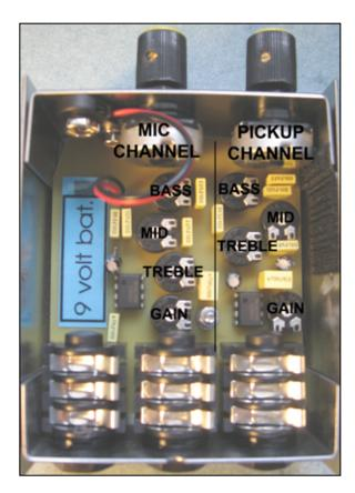
Each channel has tone controls; they have a very wide +/-20db range. Use a light touch, because a tiny tweak can make a dramatic change. Make small adjustments as necessary. After you find the best settings, we recommend you leave the settings in place and make adjustments at your amplifier to compensate for new stage and room conditions.
