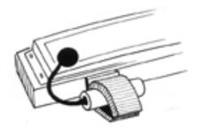
**Suggested installation for bigger harmonicas**: Inside the instrument on the reed block.
