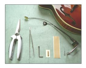
3. Apply double stick tape to the golden side of the transducers, it is a very thin film:
