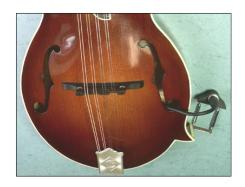
14. Bring the carpenter jack in position and use use a fitting tool (like a small Allen wrench that fits the holes in the barrel screws) to tighten the clamp as shown.
