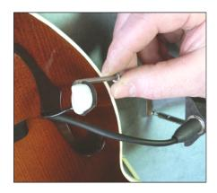
12. Remove the brown protective paper from the double stick tape on the pickup and bring the pickup into position. Use upward pressure on the installation tool to firmly press the pickup to the soundboard.
