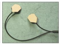
We recommend applying two layers of the double stick tape. After the first layer is applied as shown, peel off the brown protective tape. Repeat the procedure. This helps to reduce the sensitivity towards unwanted mechanical transmissions and guarantees the most secure adhesion.
