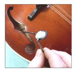
7. Remove the brown protective paper from the double stick tape on the pickup and bring the pickup into position.
