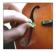
9. Use upward pressure on the installation tool to firmly press the pickup to the soundboard.
