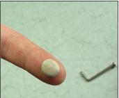
7. Stick the putty over the bent nail (your installation tool) onto the labeled-black side of the pickup. Make sure to hold the pickup so the cable leads towards the bottom of the mandolin once the pickup is attached to the soundboard. The putty will temporarily hold the pickup to the bent nail.
