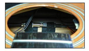
9. Attach the preamp circuit board and the battery clip to their corresponding Velcro pieces.
