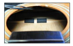
8. Plug the ¼" plug into the pickup's endpin-jack and attach the connectors to the Velcro on the brace. Make sure the cables of the pickup are looped free in the air without touching anything in your guitar.
