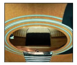
3. The preamp attaches with a peel-and-stick adhesive to the inner edge of the sound-hole (see picture). The adhesive is already attached to the unit, simply peel off the backing and attach where desired.
