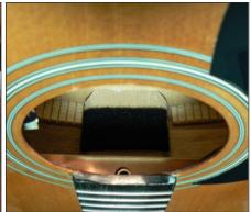
Pull the soft Velcro piece off the preamp's circuit board and stick it to the inner edge of the sound hole at the low e string side.
