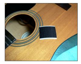
5. Stick the two pieces of hard Velcro around the second bottom brace in the lower bout of your guitar. Wrap them around the brace length-wise (so that the long side is going the same way as the brace).
