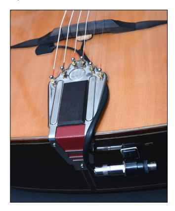
The jack mounting clip has strong double-sided tape already on it. This tape can be somewhat laborintensive to remove, so you can tape some duck tape (or similar) on the guitar first and then stick the mounting clip to the duck tape.
