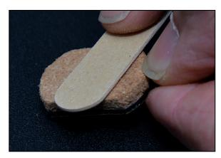
6. If the gap in your bridge is larger than the cork and you need to add height to the pickup, cut a fitting piece of a clear square or a business card and put it on top of the cork.
