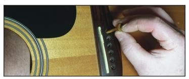
8. Guide the white pin up through the high E string hole from the inside and secure the jig by moving the golf tee to the G string hole from the outside and finding the oblong hole in the jig. This will align the jig exactly as was done in step 3, during the practice run.
