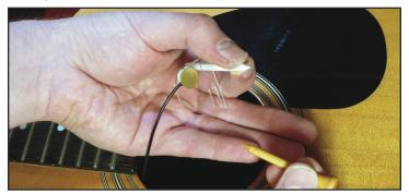
7. Move the jig inside the guitar through the soundhole. Stick the golf tee into the high E string hole from the outside with your other hand and try to feel it protruding to the inside with the thumb or index finger of your jig hand. This process helps you identify the correct pinhole on the inside.
