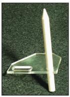
The pin should fit very snugly – you may have to use some force (or even file it down a bit) to press it into the hole. If the pin fits too loosely, please use some superglue to secure it. Wipe off excess glue and let dry.
