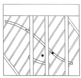
Backside of a standard piano with location of the bridges and marked positions for the three transducer heads.
