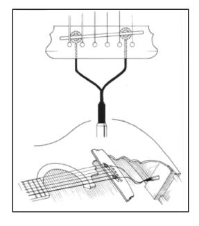
5. Unscrew the jack's endpin knob. Position endpin jack from inside the guitar into pre drilled hole. You may have to adjust the nut position to your needs. Screw endpin knob back on the jack from the outside of the instrument.
