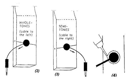
After you finished the gluing of all pickups, allow the glue to set for at least 30 minutes before you move the bars.
